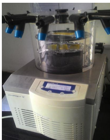
Fig. 1: Preparation of orally disintegrating films by Freeze Drying Method
