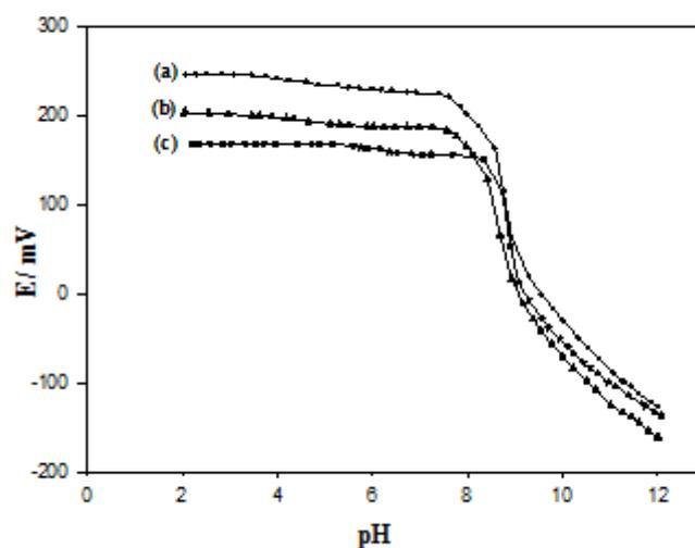
Fig. 2: Effect of pH on  $1 \times 10^{-3}$  (a),  $5 \times 10^{-4}$  (b) and  $1 \times 10^{-4}$  M CLP.HCl (c) solutions on the potential response of CLP-TPB CMCPs.
