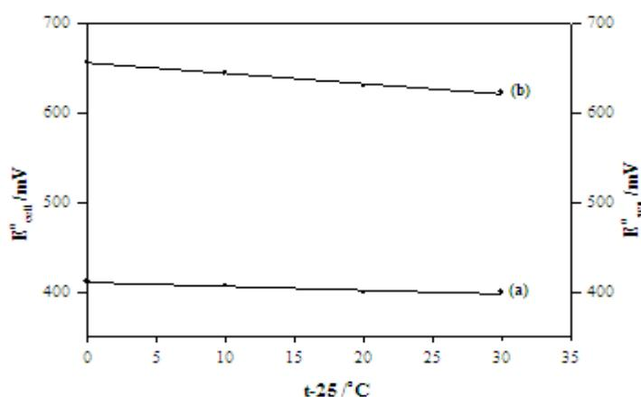
**Fig. 4: Variation of the cell standard potential (a) and the the sensor standard potential (b) of CLP-TPB CMCPs with change of test solution temperature**
