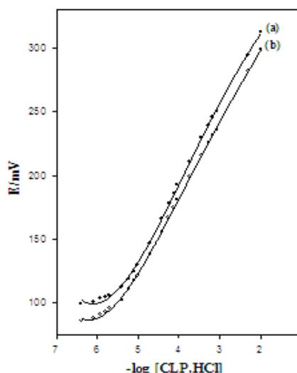
Fig. 1: Calibration curves of CLP-TPB (a) and CLP-ST CMCPSSs (b) at  $25 \pm 1.0^\circ\text{C}$
