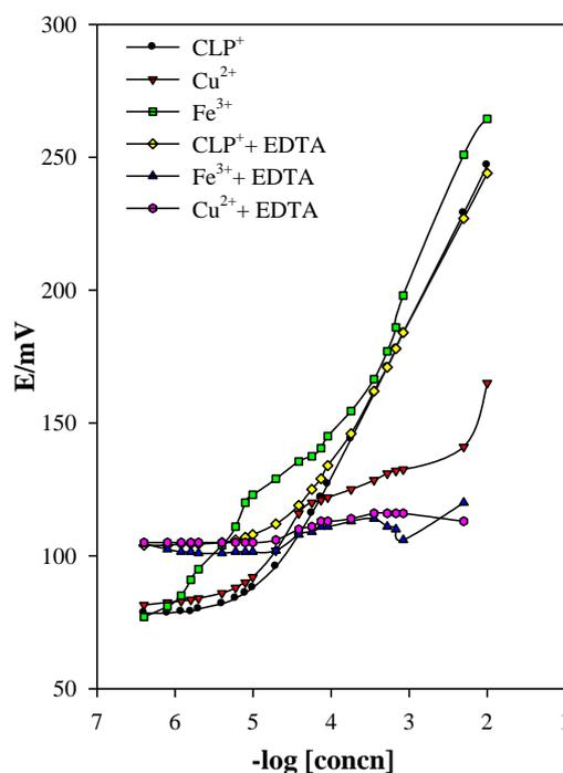
Fig. 6: Response to Fe(III) and Cu(II) in presence and absence of EDTA using CLP-TPB CMCPs
