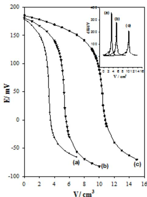
**Fig. 7: Potentiometric titration of 1.05 (a), 1.75 (b) and 3.51 mg CLP.HCl (c) against  $1.00 \times 10^{-3}$  M NaTPB using CLP-TPB CMCPSS**
