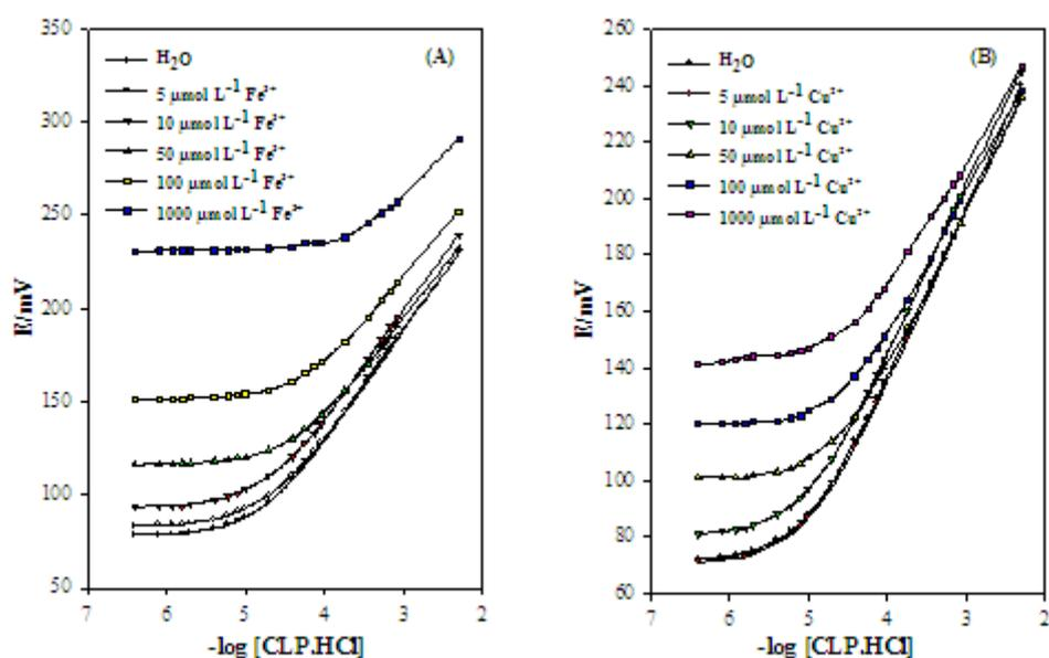
Fig. 5: Calibration graphs for CLP-TPB CMCPs at different concentrations of iron (III) (A) and copper (II) (B)
