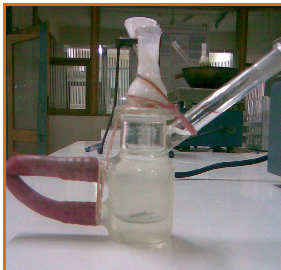
Fig. 2: Modified Franz diffusion cell used for Drug Permeation studies
