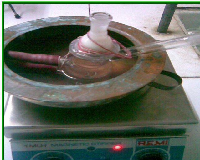
Fig. 2: Modified Franz diffusion cell used for Drug Permeation studies
